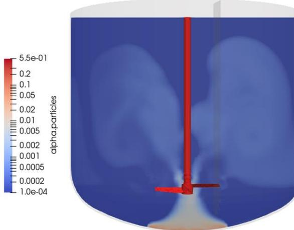
Impeller at 375 mm from bottom
