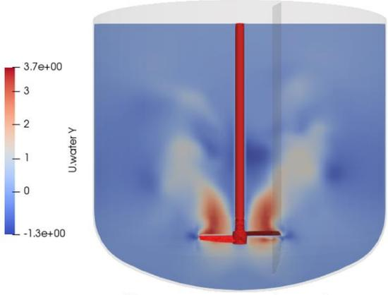
Impeller at 375 mm from bottom
