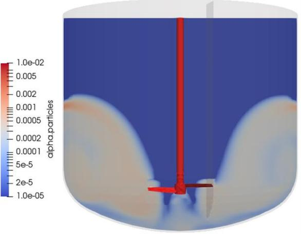
Impeller at 375 mm from bottom
