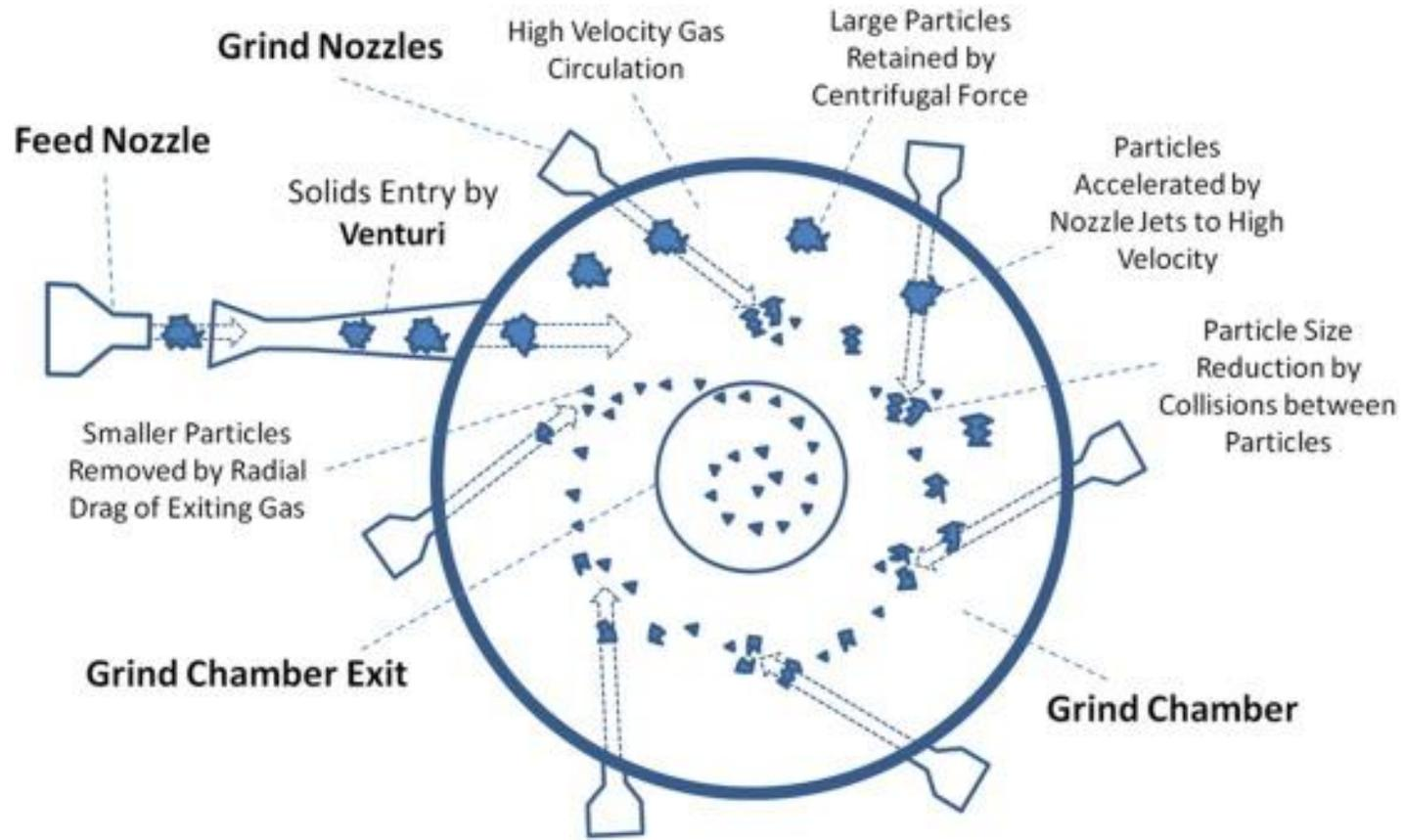
Spiral jet mill grind chamber (plan view)
