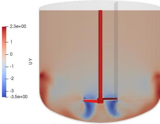
Impeller at 375 mm from bottom
