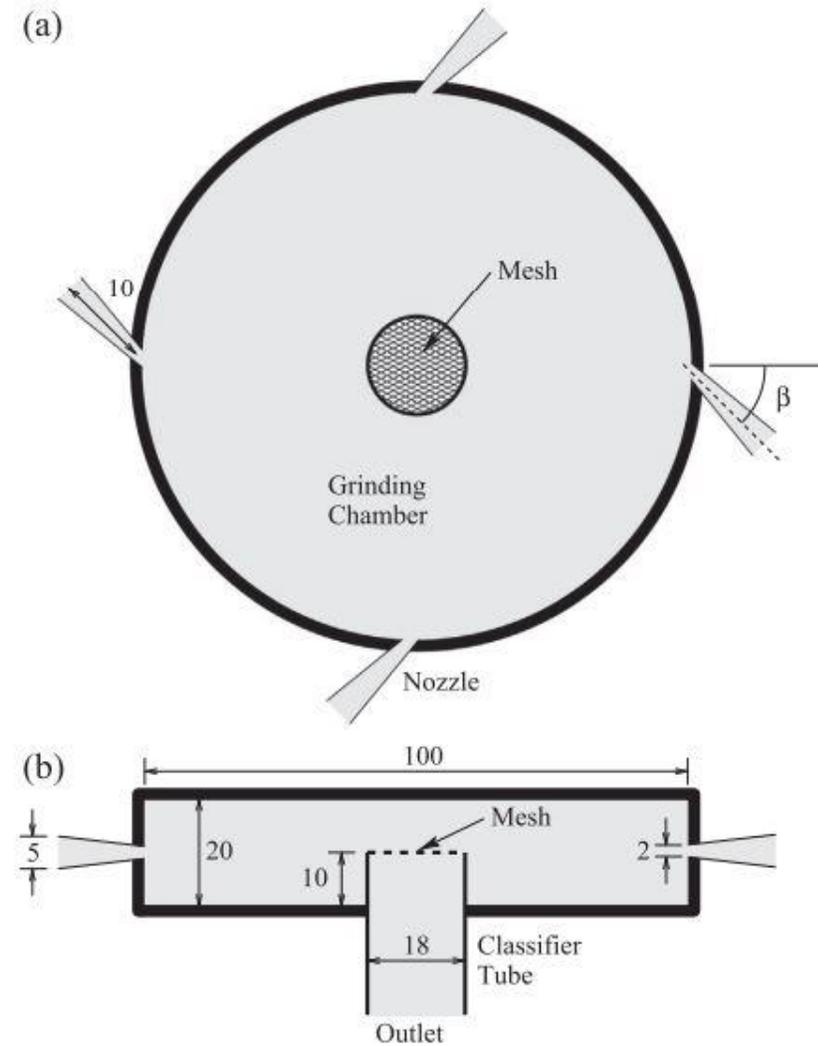
**Fig. 1.** Schematic view showing the geometry of the air jet mill used in the study. Air enters from the 4 nozzles and exits from the central classifier tube. Dimensions in mm are shown,  $\beta = 45^\circ$ . (a) Top view. (b) Side view.
